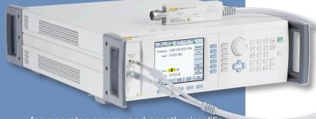
for operator errors, and greatly simplifies RF metrology. As the core of an RF and microwave calibration system, the 96040A covers the majority of test points required for calibrating spectrum analyzers of any frequency range.
